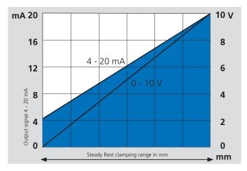
The linear stroke control unit type SCU provides a linear output signal between min. 4 mA and max. 20 mA depending on the Steady Rest clamping range.
