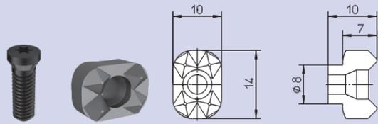
Parts included: Gripper with Torx screw
