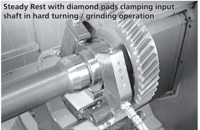
Steady Rest clamping aircraft shaft
