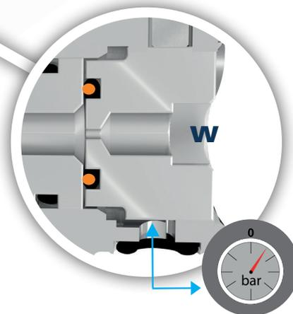
**ATTENTION:** the pneumatic system of the pressure switch must signal the alarm condition and must prevent the pallet exchange on the APS or any robot operation when the inlet pressure is less than 6 bar.
